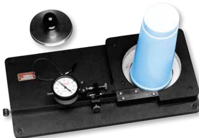
Metal band I.D. fixture for 1/2-gallon container
