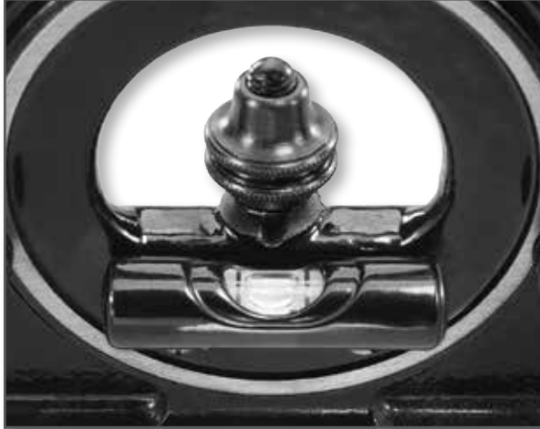
Close-up of spirit level on back side of protractor
